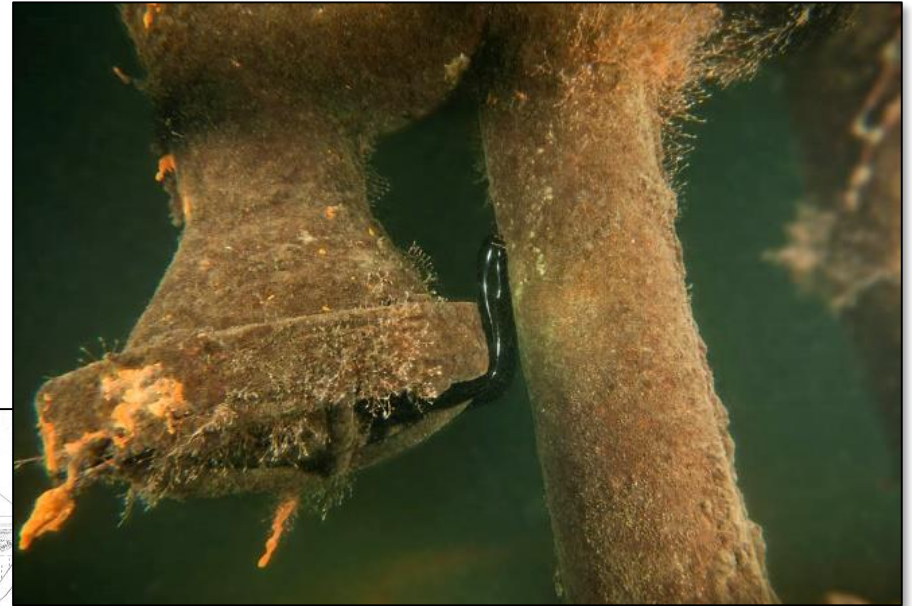
Oil from gooseneck piping, shipwreck Harburg. Swedish Coast Guard
